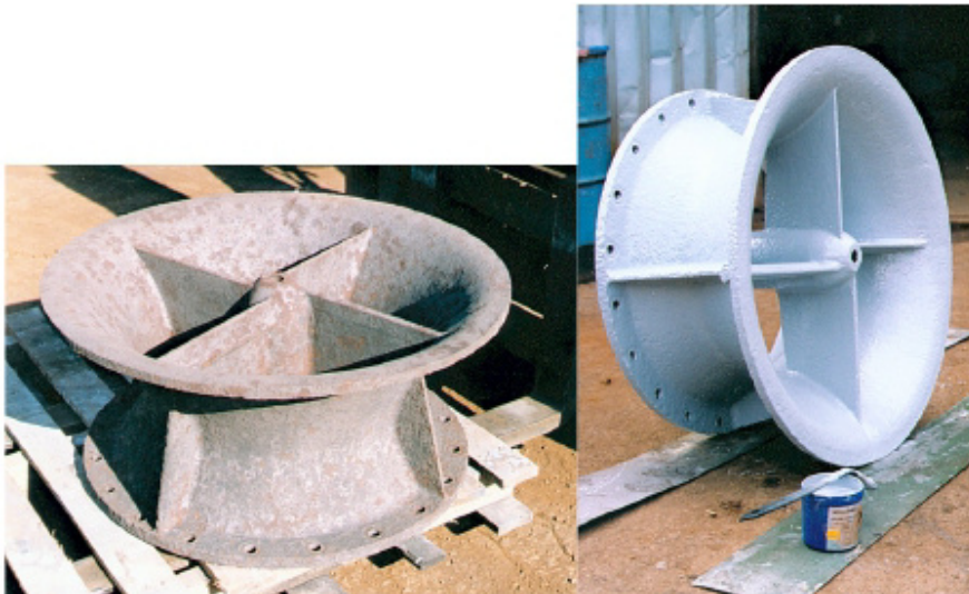
Pump Impeller blast prepared and coated with UPS 210 Super Low Friction Efficiency Coating.
