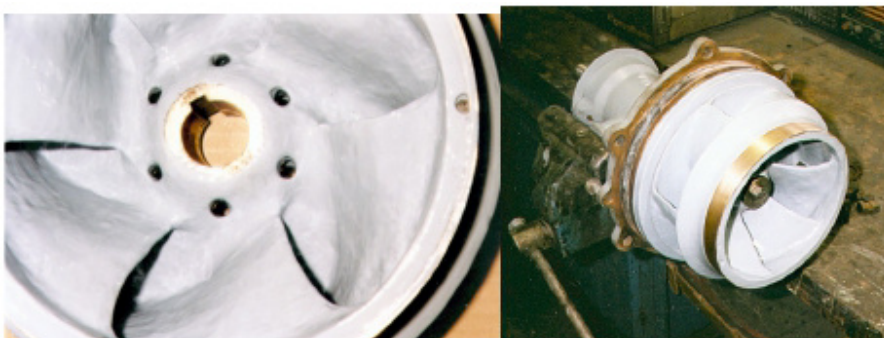
The Impeller is coated with UPS210 Super Low Friction Efficiency Coating and left to cure.
