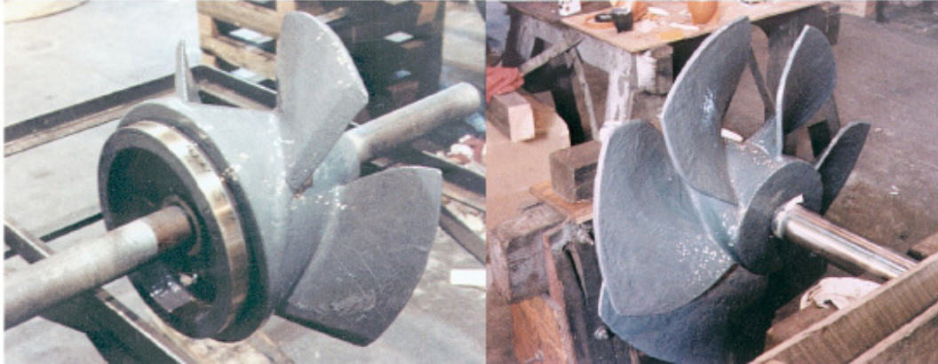
Pump Impeller blasted and cleaned with Unique Polymers Universal Cleaner and coated with UPS 210 Super Low Friction Efficiency Coating (Grey)
